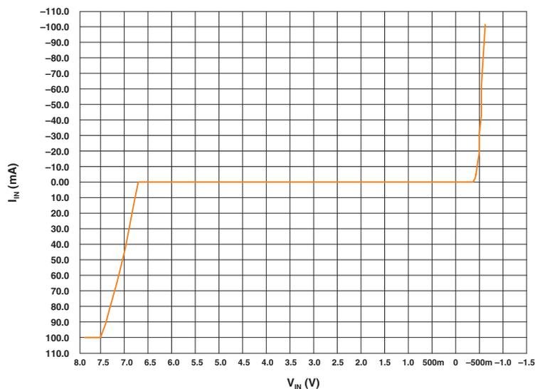
**Figure 3. Diode Current Across I/O Voltage (Typical Values)**
