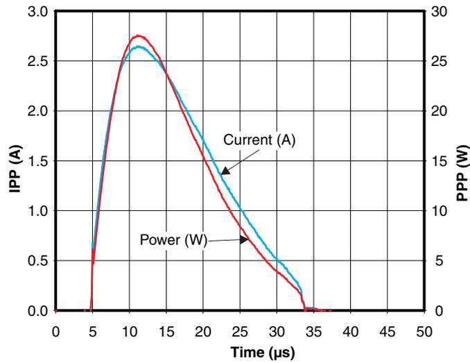
Figure 5. Pulse Waveform (8/20 µs Pulse)
