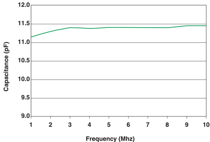
Figure 2. I/O Capacitance vs Frequency (Typical Values)
